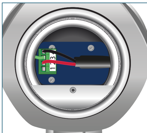
Figure 6 Terminal Block Connection
